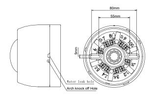
There are ten terminals with marks on the base. Only 2 of them are for connection, other will help the fixing. D1+ (9), D2- (7): Connected with I-9333 Interface, polarized
